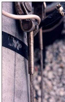
A few minutes checking swage fittings can save your rig. Look for bulging or cracks like this that signal corrosion. Replace any suspect fittings immediately.
