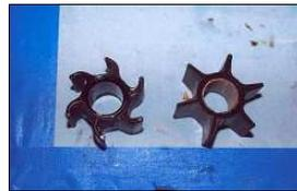
ing much easier inspection and replacement of impellers.
