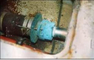
Replacing your old flax packing with a high-tech type can eliminate drips and extend the interval between changes.
