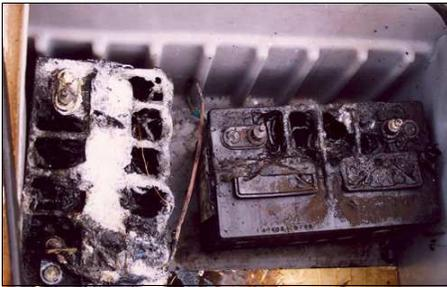
Batteries, like these conversional wet-cells, have always had the potential to start fires due to their high energy content. These caught fire when an errant wrench contacted both terminals (Claim #0205712). Newer technology batteries with higher capacities and less forgiving charging characteristics will require even more caution along with sophisticated monitoring.
